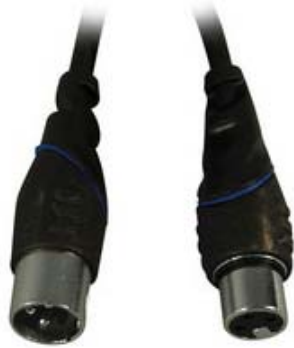
Figure-4: Mic to Preamp Cable (XLR-Female to XLR-Male connection)
